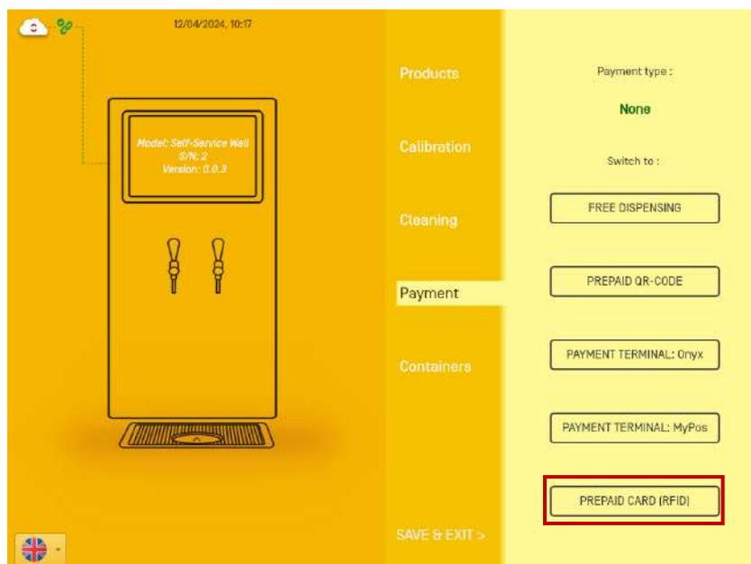
d. Check that the symbol on the screen confirms that the RFID reader is correctly connected.
