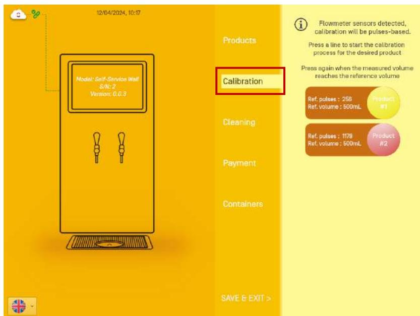
c. Press the product 1 logo once to unlock the valve and start the calibration process. Pour exactly 500mL, then press the logo again to close the valve and save the calibration
