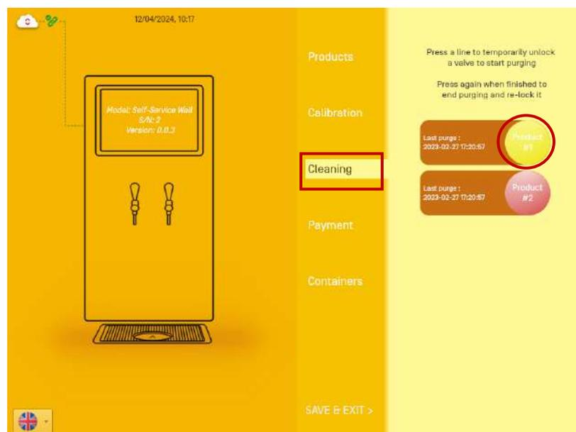
d. Replace your sanitizing solution with clear water on the line. Rinse by repeating the operation: press the logo product until the line is completely rinsed.
